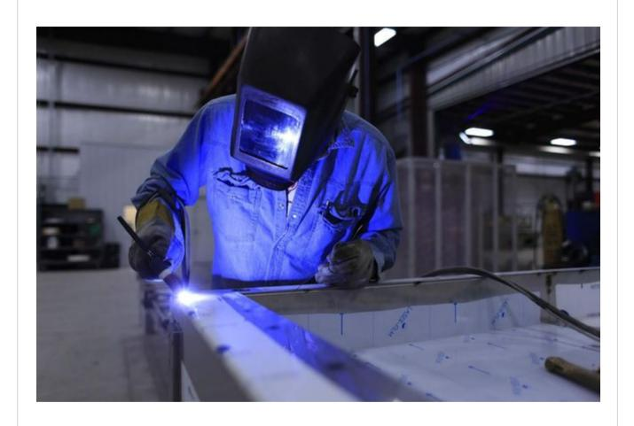
Welding is joining metal pieces or parts together by heating the surfaces to the point of melting using a blowtorch, electric arc, or other means, and uniting them by pressing, hammering, etc... There are several different types of welding techniques but the main three of the most common are Arc, MIG (Metal, Inert Gas) or GMAW (Gas, Metal Arc Welding), and TIG (Tungsten Inert Gas) welding.
